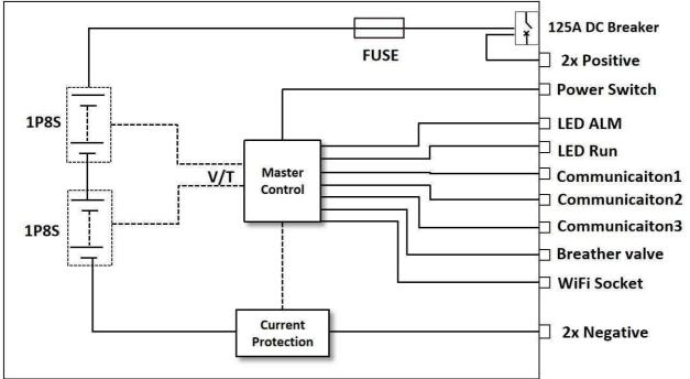
The product contains 16 lithium-ion cells in 1P16S connection, BMS PCB board, Fuse, DC breaker, MOSFET, Interconnecting wires and busbar.
