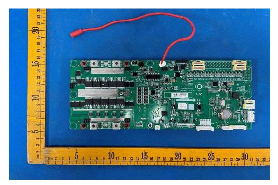
Figure 10. Front view of Main control PCB Board
